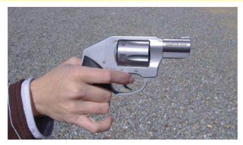
This is the Off Duty. Even in the small hands of Marie, she can only get two fingers on the grip. Charter is proud of the 3 point lock up to keep the cylinder closed. Unfortunately, the hammer drops before the cylinder actually rotates enough to locks up. This could cause a serious timing issue, something more critical than the cylinder falling open during recoil.
