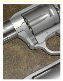
This is what I got from the factory. Look close at the marks on the frame panel and how the trigger guard slid apart. I've never seen that in a firearm before, but I have seen it looking at cars that have been in collisions.
